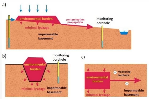
Environmental burden with zero depth of the impermeable layer a) model cross section b) front view c) top view
