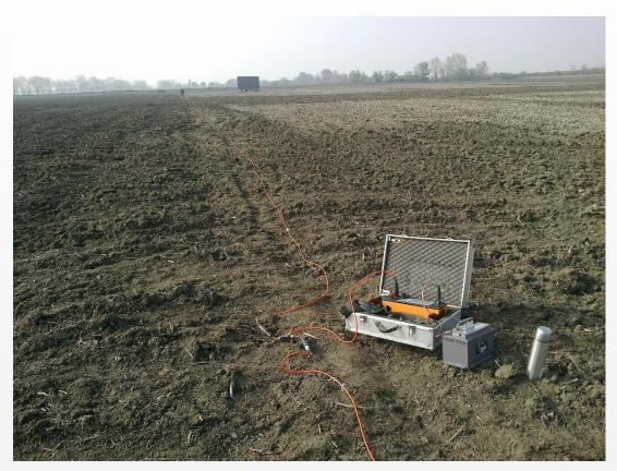
At selected profiles an electrode spacing is determined (according to target depth and resolution) and measurements are taken. This method was used at each site during this project
