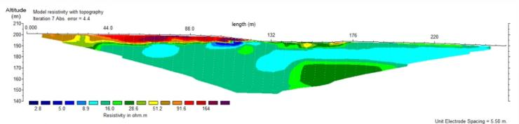
Horizontal scale is 27.34 pixels per unit spacing Vertical exaggeration in model section display = 0.60 First electrode is located at 0.0 m. Last electrode is located at 258.5 m.
