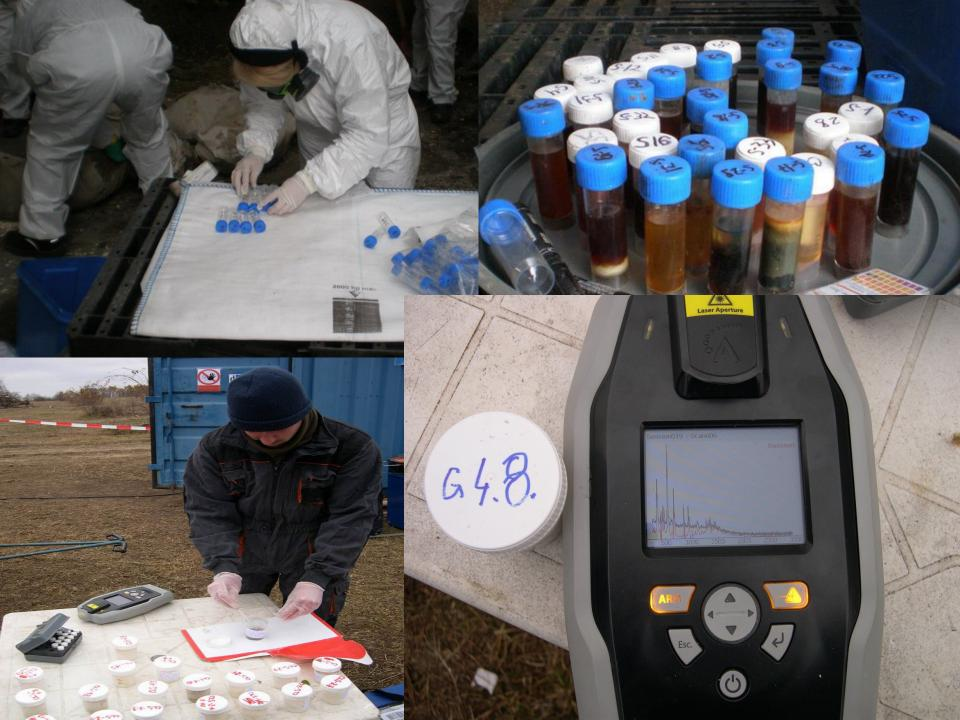
The collected samples are analyzed (Raman Spectomery) on the spot and taken to our on site mobile laboratory where they are analyzed
