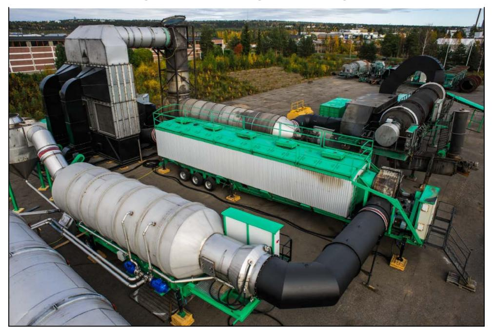
**SAVATERRA Oy - 14. Gas scrubber** is connected to process if sulphur ( $SO_x$ ) concentration in soil or fuel is exceptional high level.  $SO_x$  will react with water and sodium hydroxide as follows:
