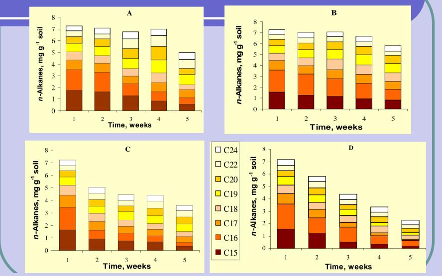
Soil systems: A – control (no additions); B – non-inoculated sawdust; C – immobilized *Rhodococcus* cells; D –immobilized *Rhodococcus* + biosurfactant
