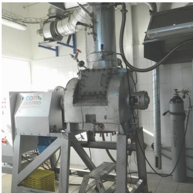
**Fig. 2.**Mixed dryer of semi-pilot testing unit.
