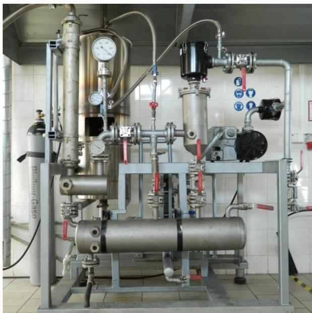
**Fig. 3.** Condensation unit of semi-pilot testing unit.
