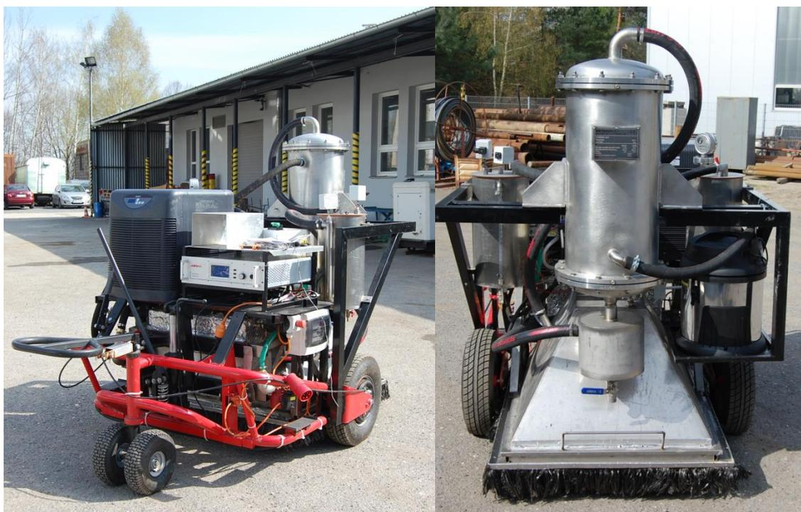
**Fig. 2.** VLNOCHOD Microwave remediation device
