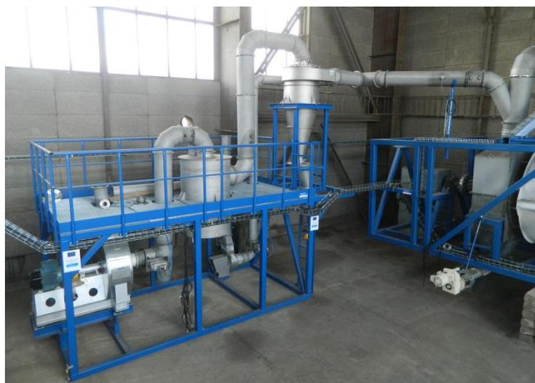
**Fig. 5.** Off-gas pretreatment module of continuous thermal desorption pilot unit.
