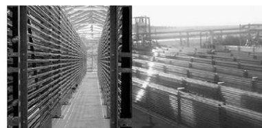
Figure.4 Closed systems for growing algae
