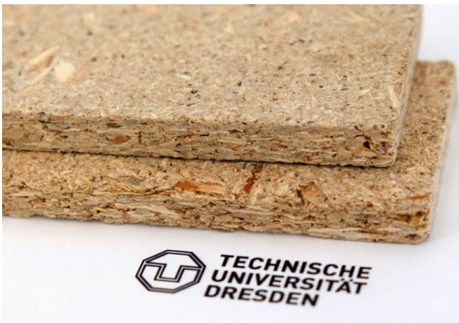
Figure 3. Particle board produced from Miscanthus biomass cultivated at the land field
