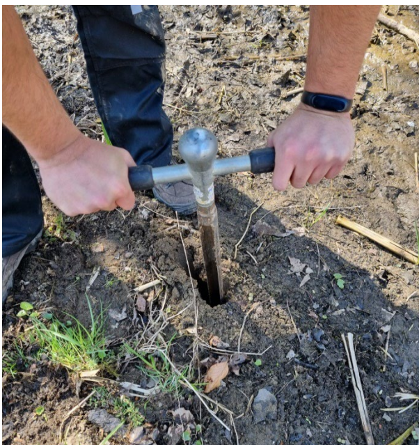
Figure 1. Taking a sediment sample using a hand sampler
