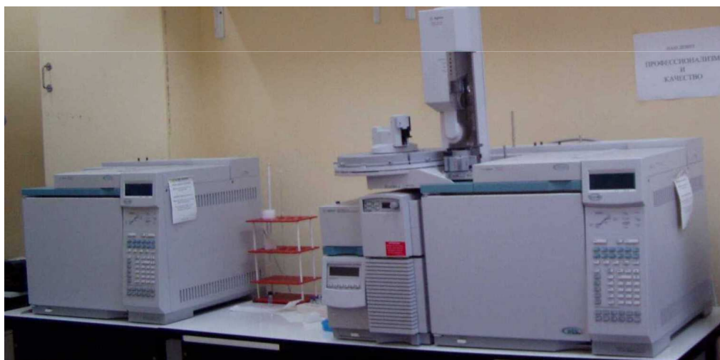
Gas Chromatograph Agilent6890 (2000) equipped by \mu ECD and FID detectors. Gas Chromatograph with Mass Selective detector Agilent6890/5973
